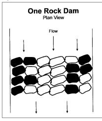
can be accomplished by placing larger rocks in the deepest part of the channel, smaller ones to either side. (Figure 12.) Do not stack rocks on top of one another to get the needed height. The stacked rocks will be swept away by flood flows. Placing greatly oversized rocks in the structure will generate turbulence that could undermine it. Rocks should be sized propor-
