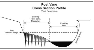
When a series of structures is installed at appropriately spaced intervals, materials eroded from the concave bank, opposite one deflector, will tend to be deposited adjacent to or on top of the next downstream deflector, thus forming a convex bank. These deposited materials are soon stabilized by encroaching streambank vegetation and a new floodplain evolves where none existed before (Figure 6).
