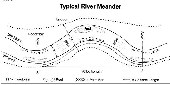
ficient space for a meandering channel to reach its equilibrium meander amplitude. Similarly, it would be inappropriate to modify a dynamically stable channel by attempting to increase its width, flatten its slope, or increase its sinuosity because such alterations would interfere with the ability of the stream to accommodate flood flows or transport its bedload.
