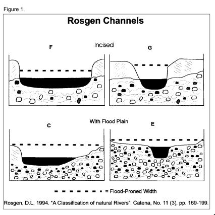
to watershed equilibrium, incised channels will tend to widen (due to lateral erosion of their banks), flatten, become more sinuous, and develop a meander pattern along with floodplain characteristics similar to the pre-disturbance condition. In other words, disturbed channels tend to evolve toward a state of dynamic stability appropriate to watershed geology, sediment
