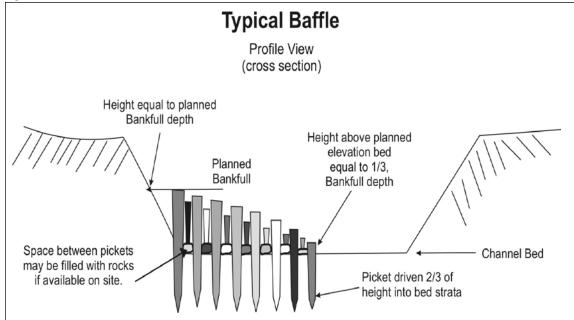
When choosing between rocks or pickets as baffle-making material, pickets are more appropriate to clay, sand, or gravel bedded channels while rocks are more appropriate to cobble or boulderbedded channels. Rock baffles are especially appropriate to smaller, steeper ephemeral and intermittent streams and arroyos, where the properly sized materials are usually readily available and driving pickets is difficult.
