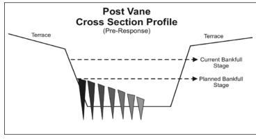
However, the receding bank resists erosion to Figure 6. some degree depending on its stability and repels the concentrated flow. The repelled flow then rebounds toward mid-channel, gradually crossing over and impinging on the other bank. In other words, a baffle installed on the left bank will deflect flows toward the right bank only to be rebounded again toward the left bank farther downstream.
