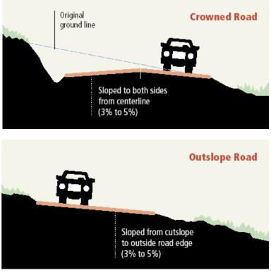
Outsloping, grade dips, open top culverts, and/or water bars can drain roads constructed on moderate slopes with light traffic loads. Though inexpensive to install, these methods may require frequent maintenance during periods of heavy use. This drainage method is not recommended on steep slopes or unstable soils for reasons of stability, safety and maintenance problems.
