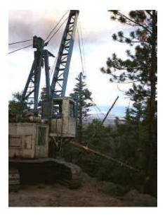
They are typically used on slopes 40-100%, and with yarding distances up to 5000 feet. Aerial logging systems are also used for high-value selective logging and in areas where the appearance of the landscape is especially important.
