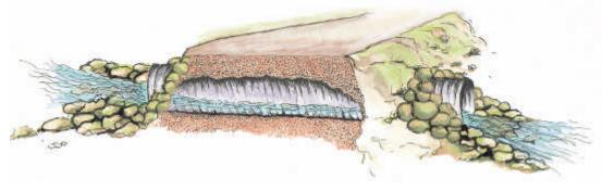
Align the culvert exactly with the stream, on the existing grade, and at the depth of the streambed. The
