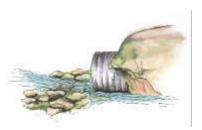
direction of the stream flow even slightly, there will be increased channel erosion. If a culvert is installed at a steeper grade than the stream, it will accelerate the flow and cause erosion at the outlet. However, the grade must be steep enough to prevent sedimentation in the culvert.
