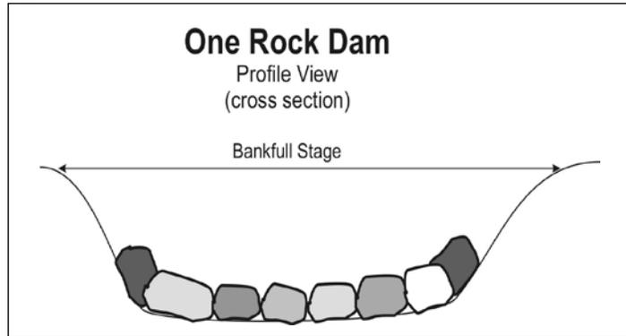
***Weirs establish bed elevation and channel slope gradient.***
