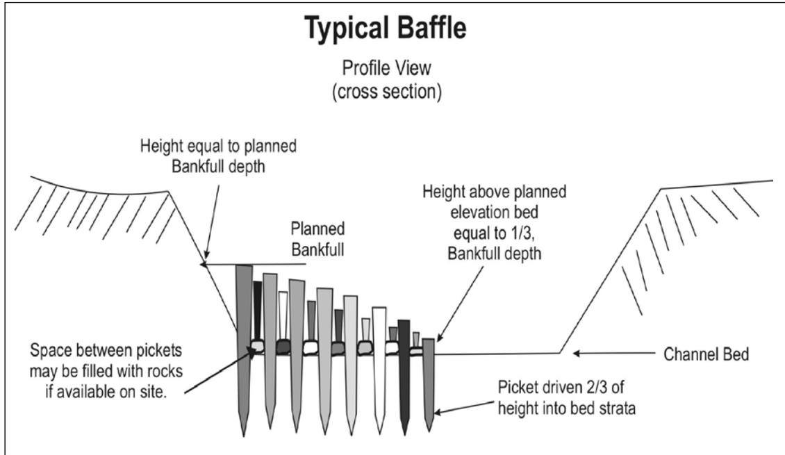
require about 30-50 pickets. Whether built of rock or pickets, the height of the baffle should taper down from bankfull to a mid-channel height of about 1/3 bankfull. It is easier to cut pickets at the appropriate height above the channel bed than to drive them to appropriate height.
