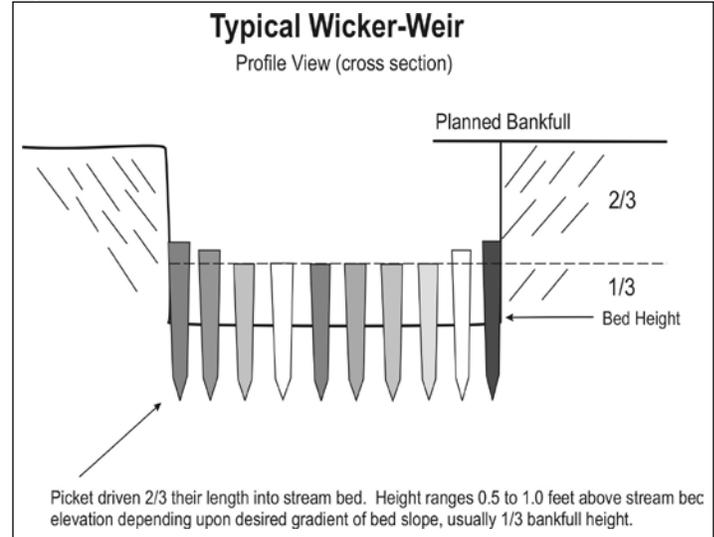
down will prevent sprouting. Wicker weirs can be reinforced with the use of wicker materials woven between the stakes and are installed midway between baffles, and placed at an angle to anticipate the future course that the water will flow (see photos on front cover).
