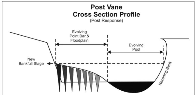
When a series of structures is installed at appropriately spaced intervals, materials eroded from the concave bank, opposite one deflector, will tend to be deposited adjacent to or on top of the next downstream deflector, thus forming a convex bank. These deposited materials are soon stabilized by encroaching streambank vegetation and a new floodplain evolves where none existed before (Figure 6).
