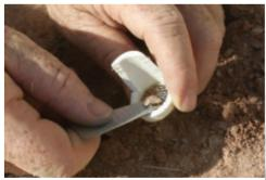
Figure 4. Place sample in sieve.
