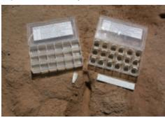
**Figure 5.** Complete soil stability kit with water and samples.
