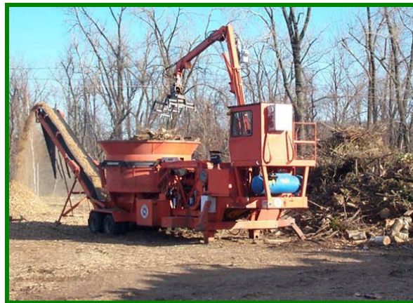
Photo 3 – Community wood trimmings being ground into chips using a tub style grinder.
