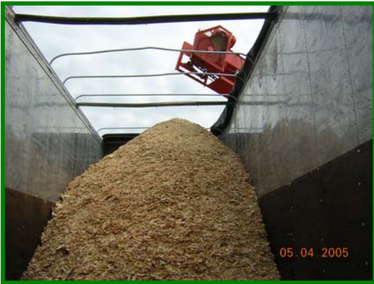
Photo 2 – Dowler chips conveyed directly into a live bottom trailer at a post and pole mill.
