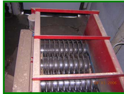
Photo 7 – Sizing equipment used for removing over-sized chips at a wood-chip heating facility.
