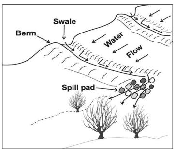
capture runoff and make it soak in the soil. Swales and berms work best on well-drained, sandy and loamy soils in conjunction with other soil conservation and water harvesting techniques. On clayey soils infiltration is too slow, which may cause swales to overflow and breach, which exacerbates the erosion we intend to stem. Swales and berms are labor intensive to install and need
