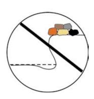
A futile treatment is to pile rock or other materials on the top of the headcut in the belief that doing so will protect the lip from erosion. Since headcuts advance with the progressive undercutting and collapse of the headwall, this treatment will not succeed. In fact, raising the lip only serves to increase the erosive energy of the water falling from a greater height.
