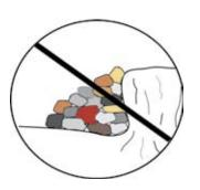
Another futile treatment is to pile loose rock at the base of the headwall on the assumption that the rocks will blunt the force of the falling water, stopping the headcut. While this treatment works initially, a space will gradually open along the face of the cut due to drying and crumbling of
