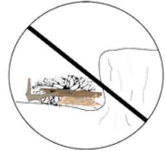
Piling brush at the face of the cut is sometimes effective, sometimes not, depending on the height of the cut and the nature of the substrate. Brush may trap other debris, thus mulching the site, keeping it moist and encouraging revegetation, but more often than not the cut will continue to move headward.
