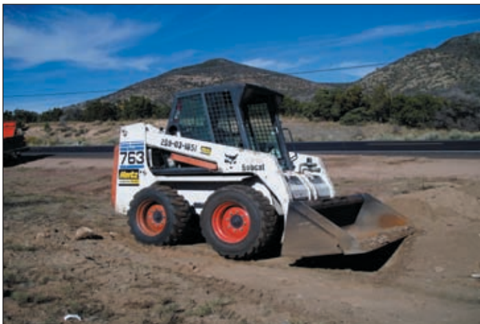
Photo IX-3: Skid -steer units are relatively cheap, adaptable and easy to transport from site to site.
