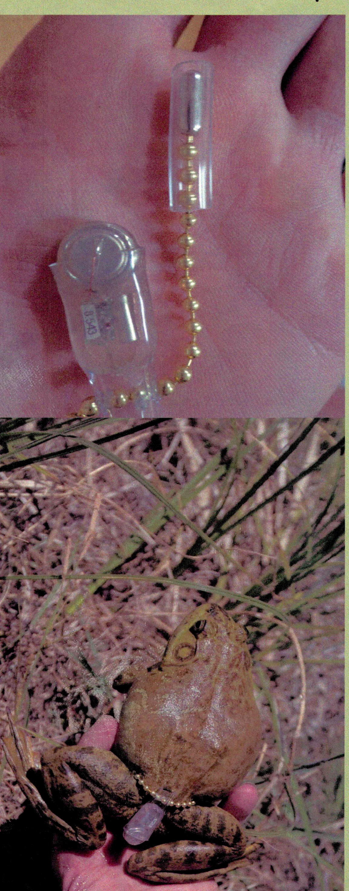
Figure 1. Left, Temperature sensitive radio transmitter and plastic tubing and beaded copper chain. Right, radio transmitter attached to bullfrog about to be released.
