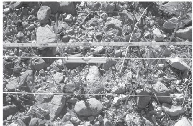
**Figure 14.2.** Level the string across the channel.
