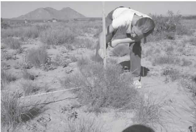
**Figure 15.1.** Line-point intercept with height alternative.
