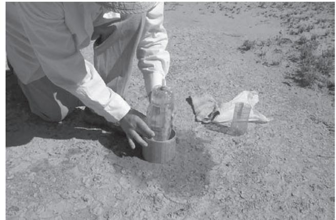
Figure 8.7. Suspend bottle inside the ring.
