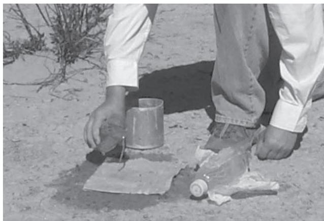
**Figure 8.3.** Pre-wet the soil to a 4 cm depth.
