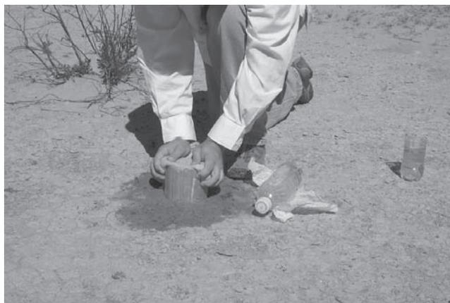
**Figure 8.4.** Insert infiltration ring to 3 cm.
