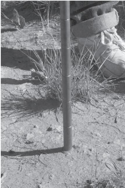
**Figure 7.3.** The top of the cone is flush with the soil surface.
