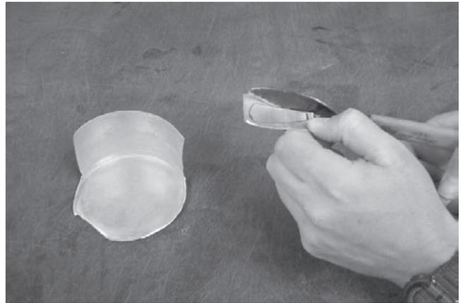
**Figure A.5.** Cutting shovels with tin snips.
