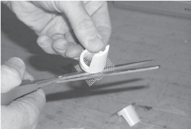
**Figure A.4.** Cutting out baskets from screen.
