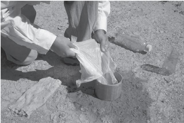
Figure 8.5. Add 370 ml water, using plastic sheet.
