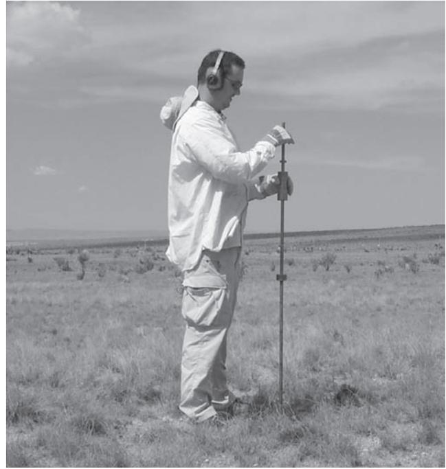
**Figure 7.1.** Impact penetrometer with sliding hammer elevated.
