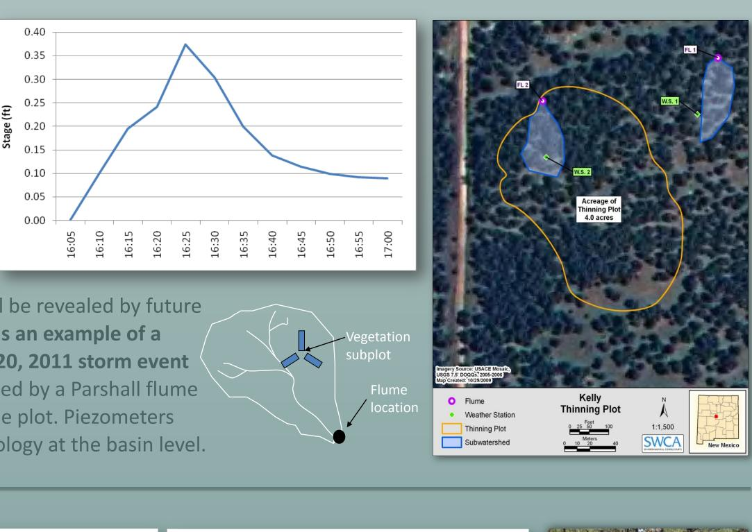
these differences persist, and for how long will be revealed by future monitoring of flow events. The graph at right is an example of a flow event which occurred during an August 20, 2011 storm event at the treated Chilili site. This flow was recorded by a Parshall flume located at the base of the subwatershed for the plot. Piezometers and wells are also being used to monitor hydrology at the basin level.
