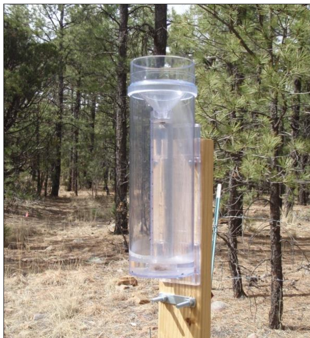
Figure 2.8. Graduated rain gauges are used for backup in the case of failure of one of the WatchDog weather stations.
