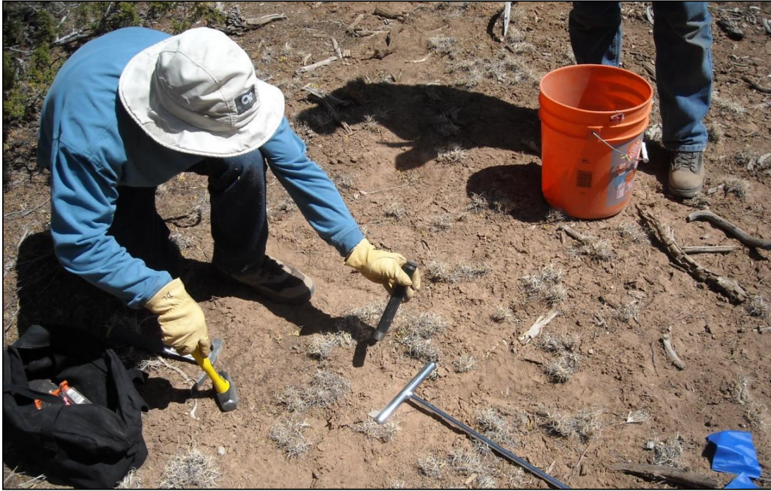
Figure 2.29. Soil cores were taken using an impact corer, shown above, for chemical analysis.
