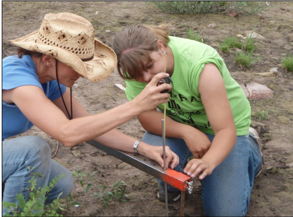
Figure 2.23. Measurement of soil surface topography using a soil movement bridge helps understand the yearly variability associated with soil topography.
