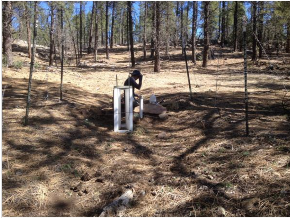
Figure 2.38. Parshall flume located at the thinned Chilili site.
