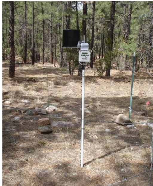
Figure 2.1. WatchDog weather station at the Westponderosa pine site.
