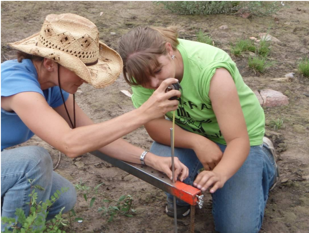
Figure 2.21. Measurement of soil surface topography using a soil movement bridge helps understand the yearly variability associated with soil topography.
