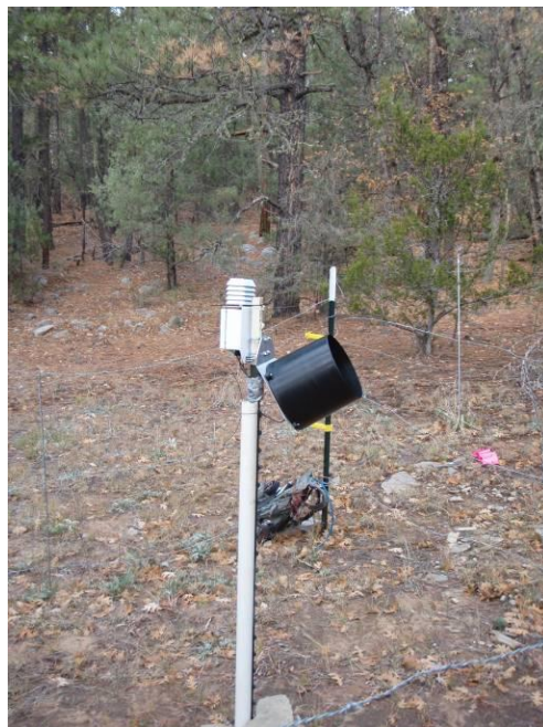
Figure 2.7. Photo taken October 27, 2009, at the Chilili ponderosa pine site showing bear damage to the precipitation bucket causing precipitation not to be recorded.
