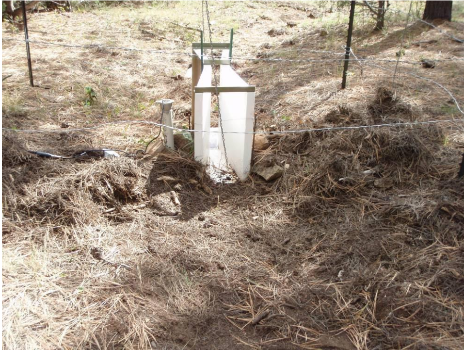
Figure 2.29. Parshall flume located at Chilili site plot 1.
