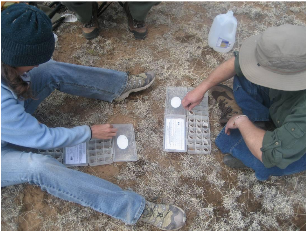
Figure 2.18. Soil stability test in use on the study sites.
