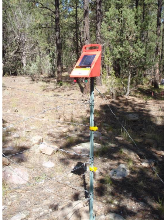
Figure 2.6. Charging station for the electric fence constructed around the WatchDog station at the Chilili ponderosa pine study site in 2009 to combat the bear problems.
