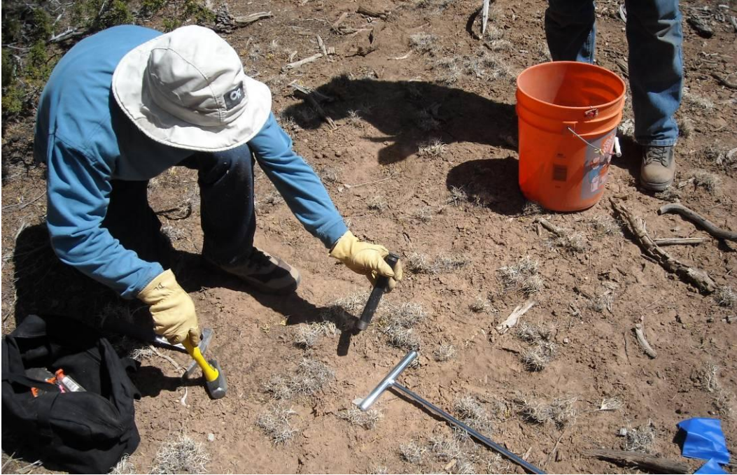
Figure 2.23. Soil cores were taken using an impact corer, shown above, for chemical analysis.
