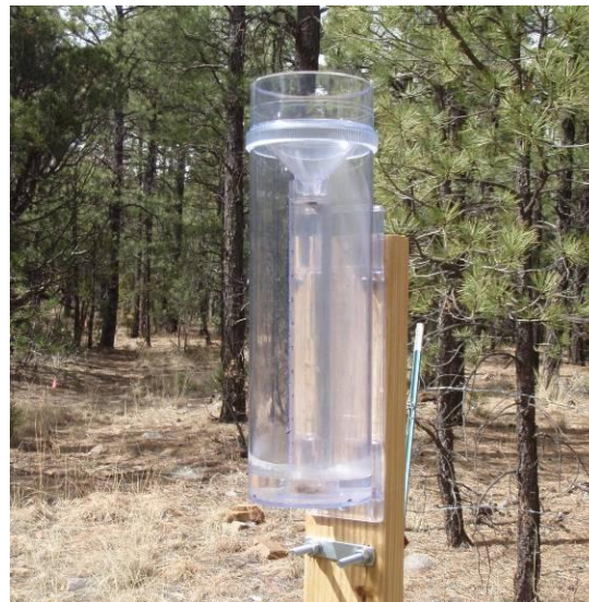
Figure 2.2. Graduated rain gauges are used for backup in the case of failure from one of the WatchDog weather stations.
