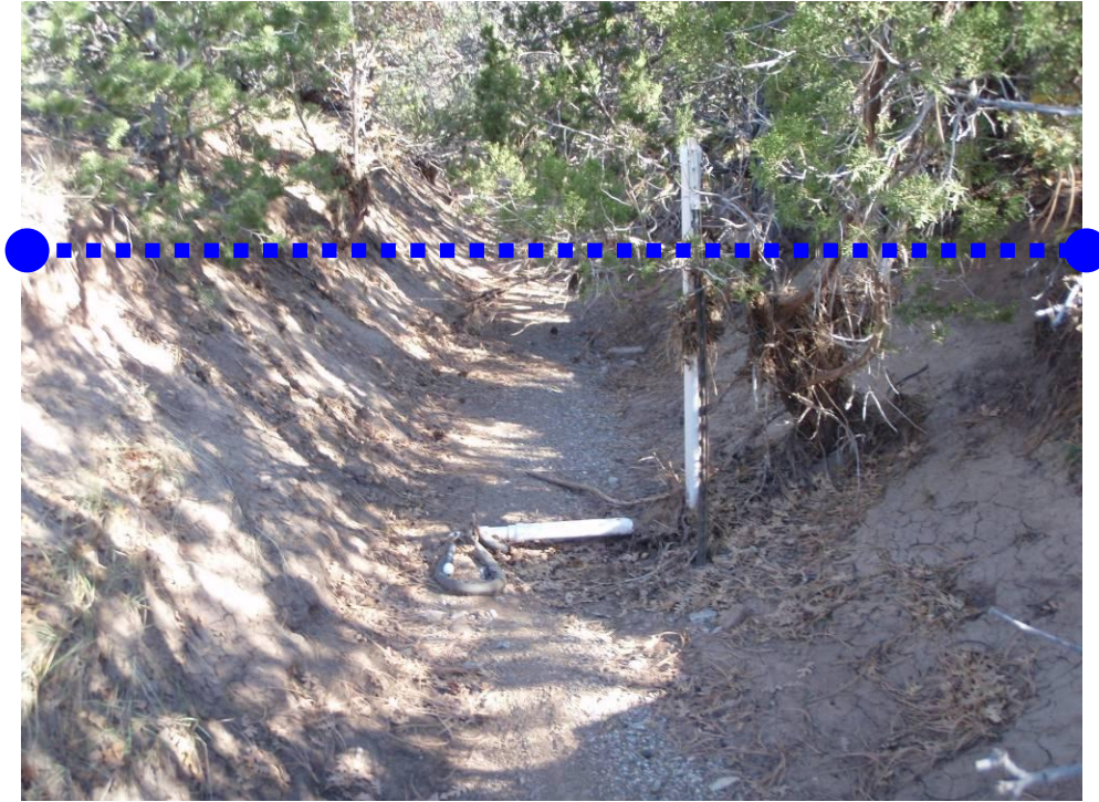
Figure 4.6. The Vigil piezometer in the fall of 2009 after a storm event lowered the stream bed level to below the piezometer. The blue line represents the high water line determined by the accumulation of debris in the vegetation.
