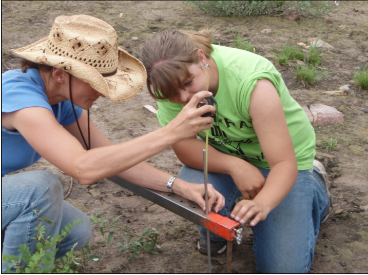
Figure 2.33. Measurement of soil surface topography using a soil movement bridge helps understand the yearly variability associated with soil topography.
