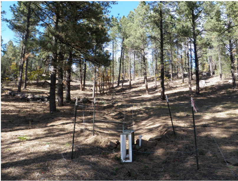
Figure 2.48. Parshall flume located at the thinned Chilili site.
