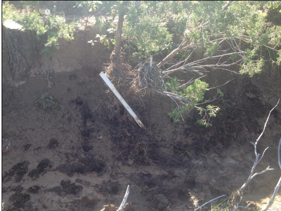
**Figure 3.2.** The Vigil piezometer in the fall of 2013 after a storm event compromised the gauge.
