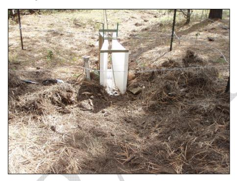
Figure 2.38. Parshall flume located at the thinned Chilili site.
