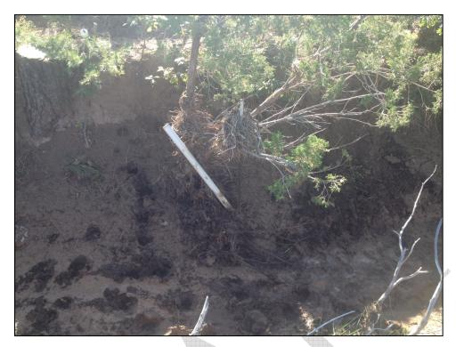
Figure 3.2. The Vigil piezometer in the fall of 2013 after a storm event compromised the gauge.
