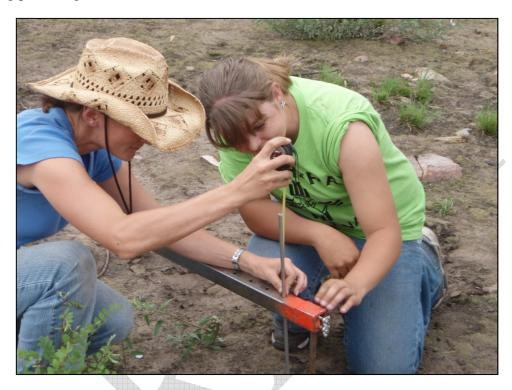
Figure 2.23. Measurement of soil surface topography using a soil movement bridge helps understand the yearly variability associated with soil topography.
