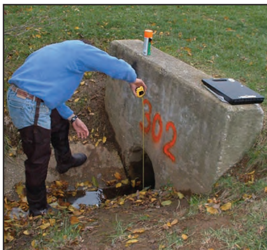
Figure 27: Measuring Outfall Diameter
