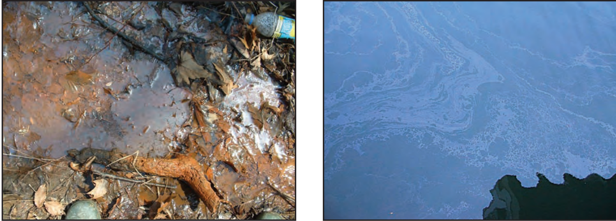
Figure 36: Synthetic versus Natural Sheen (a) Sheen from bacteria such as iron floc forms a sheet-like film that cracks if disturbed (b) Synthetic oil forms a swirling pattern
