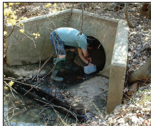
Figure 30: Measuring flow (as volume per time)
