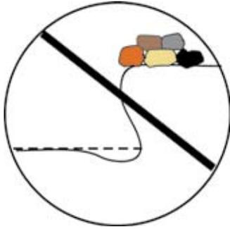
A futile treatment is to pile rock or other materials on the top of the headcut in the belief that doing so will protect the lip from erosion. Since headcuts advance with the progressive undercutting and collapse of the headwall, this treatment will not succeed. In fact, raising the lip only serves to increase the erosive energy of the water falling from a greater height.
