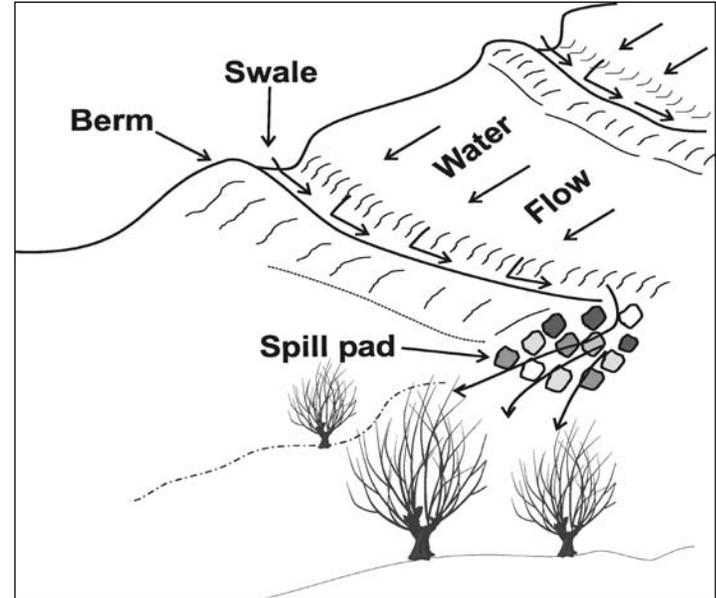
capture runoff and make it soak in the soil. Swales and berms work best on well-drained, sandy and loamy soils in conjunction with other soil conservation and water harvesting techniques. On clayey soils infiltration is too slow, which may cause swales to overflow and breach, which exacerbates the erosion we intend to stem. Swales and berms are labor intensive to install and need
