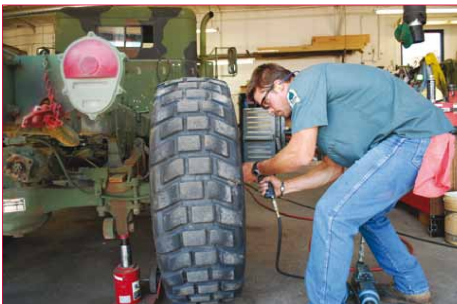
Colorado State Forest Service mechanic Nate Taggatz removes a tire during a truck overhaul.
