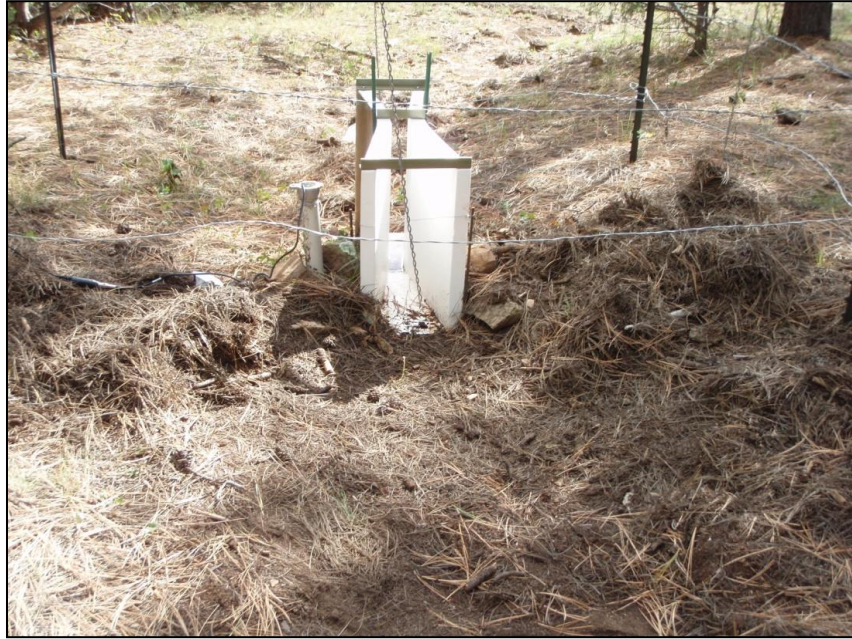
Figure 2.47. Parshall flume located at the thinned Chilili site.
