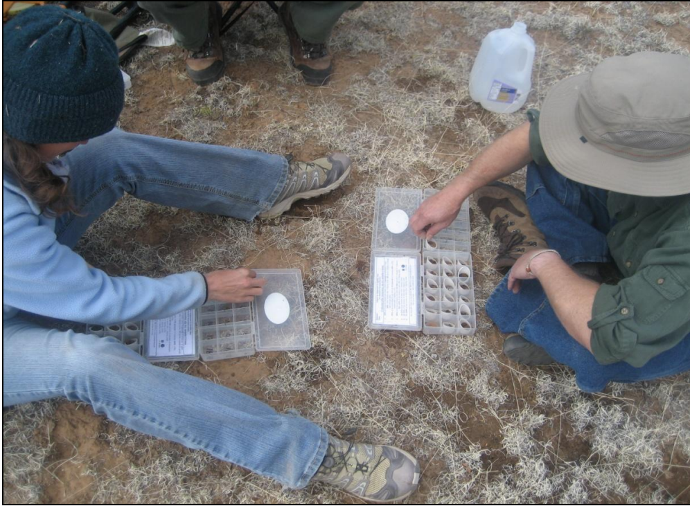
Figure 2.21. Soil stability test in use on the study sites.
