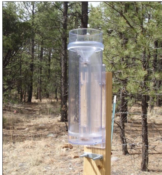
Figure 2.6. Graduated rain gauges are used for backup in the case of failure from one of the WatchDog weather stations.
