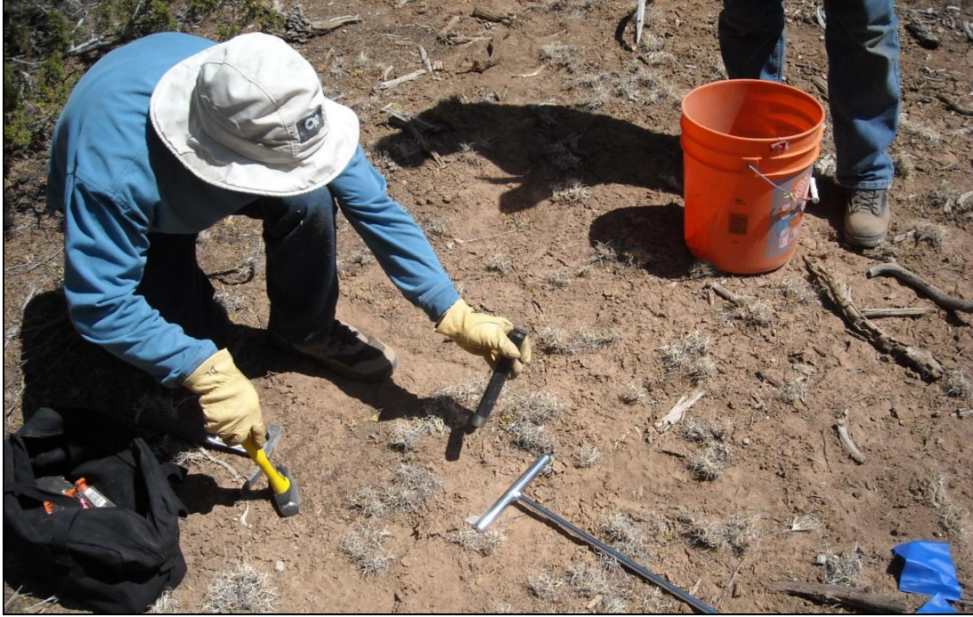
Figure 2.38. Soil cores were taken using an impact corer, shown above, for chemical analysis.
